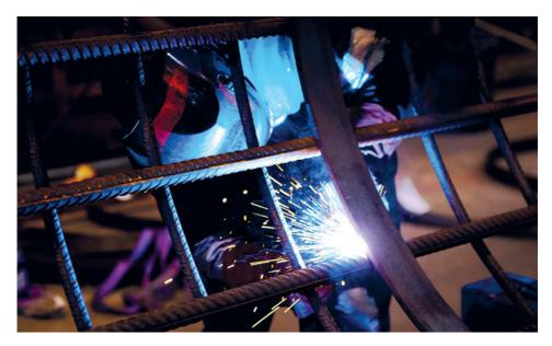
The use of factory welded prefabricated reinforcement is increasing as designers, engineers and contractors realise the benefits that prefabrication can make towards improving on-site productivity. Typical pre-assembled units include:
