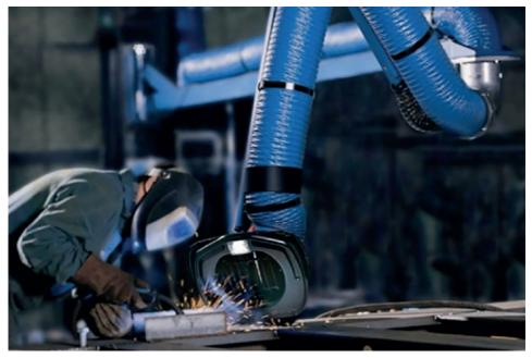
LEV systems suck and remove the welding fume and gases away from the breathing area.
