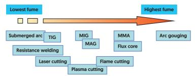
Wherever practicable a fabricator should select the welding technique that produces the least amount of fume, although just like any process the set up of the welding equipment affects the amount of fume produced, such as excess current and long duty cycles.
